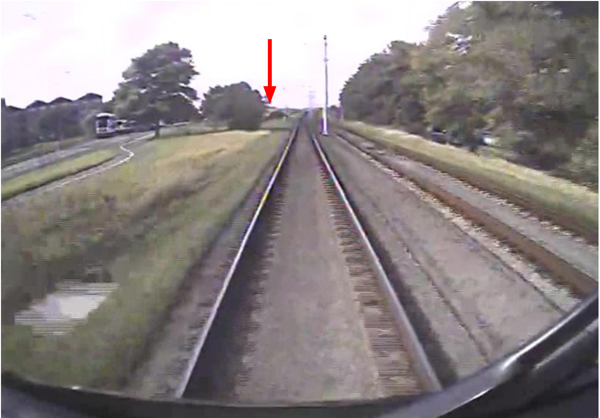
Figure 4: Image from the FFCCTV of tram 260 at around 73 metres from the crossing and 4.6 seconds before the collision. The arrow indicates the location from which the pedestrian emerges very shortly afterwards.
