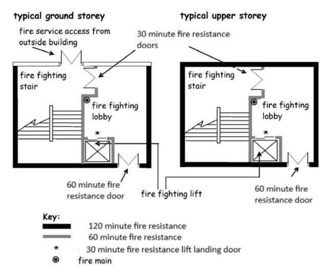
Figure 8 Fire-fighting shaft arrangement showing fire resistance ratings
