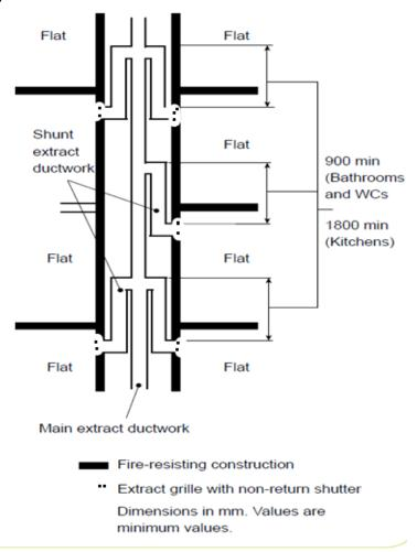
Figure 2 – Shunt duct arrangement
